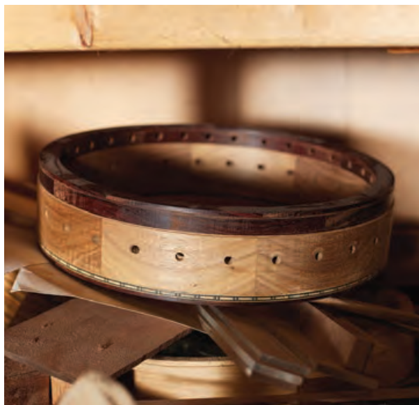
LEFT Detail of a custom-inlaid headstock on a Getman banjo. BELOW Forming a perfectly round rim is part of the time-consuming process of constructing a banjo.
